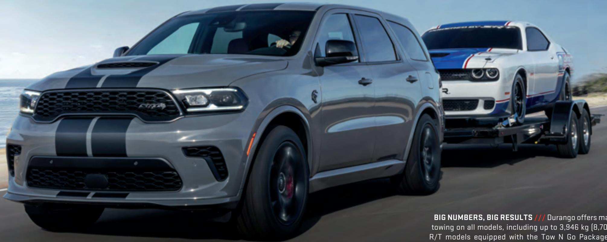
**BIG NUMBERS, BIG RESULTS** /// Durango offers mammoth towing on all models, including up to 3,946 kg (8,700 lb) on R/T models equipped with the Tow N Go Package. Outfit Durango with the available 360-horsepower 5.7L HEMI V8 engine and available Trailer Tow Group for up to 3,226 kg (7,200 lb) of towing. Models equipped with the 3.6L Pentastar V6 engine can tow up to an impressive 2,812 kg (6,200 lb).
